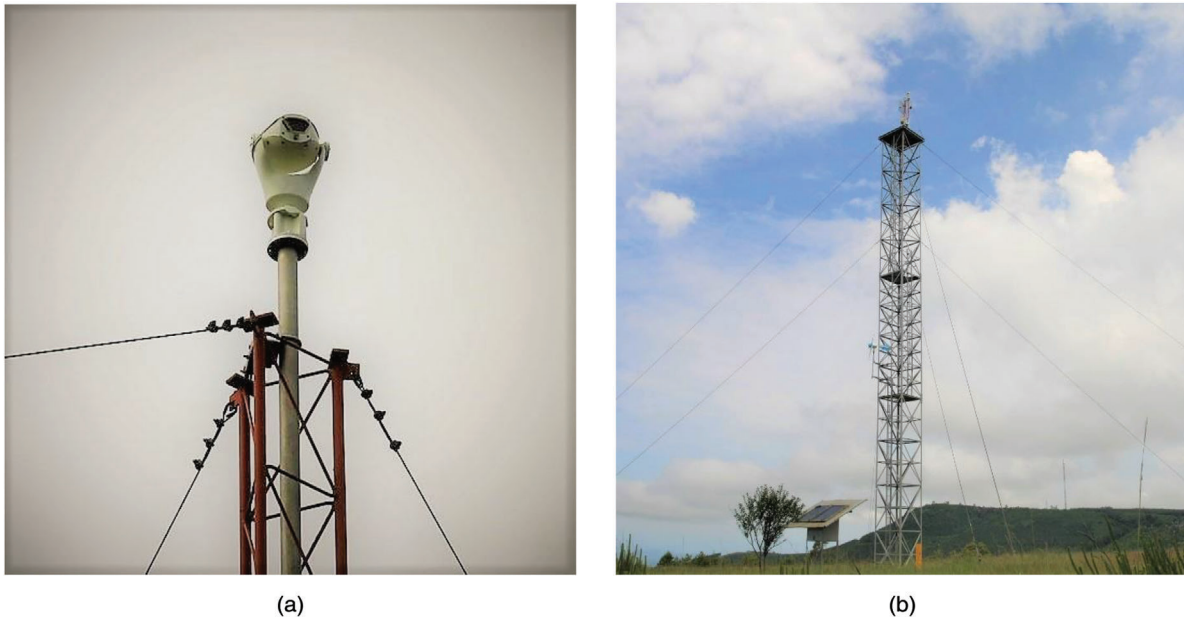
Fig. 1. (a) Camera used in a CWDS; (b) a 32-m tower on top of which a camera is placed, with the solar power supply visible near the base of the tower (Heyns et al., 2019).
